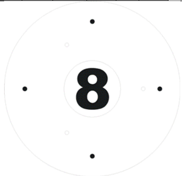
Pattern 8 – 4 Segment Brooms – 36 Inches Elgin Air Cub, Elgin Crosswind, Elgin Pelican Tymco 210, Tymco 300, Tymco 435 Schwarze A4000 Leach Vac – all Masco LH2000 Sweeprite Husky
